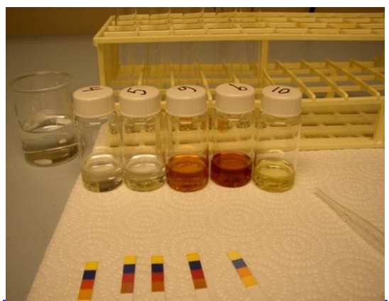
Figure 1. Stability tests comparing basic DMSO formulas (Left vials=clear solutions) to other solvent blends.
